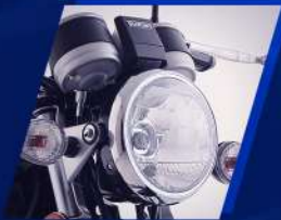
35 watt bulb in the head light for brighter light
